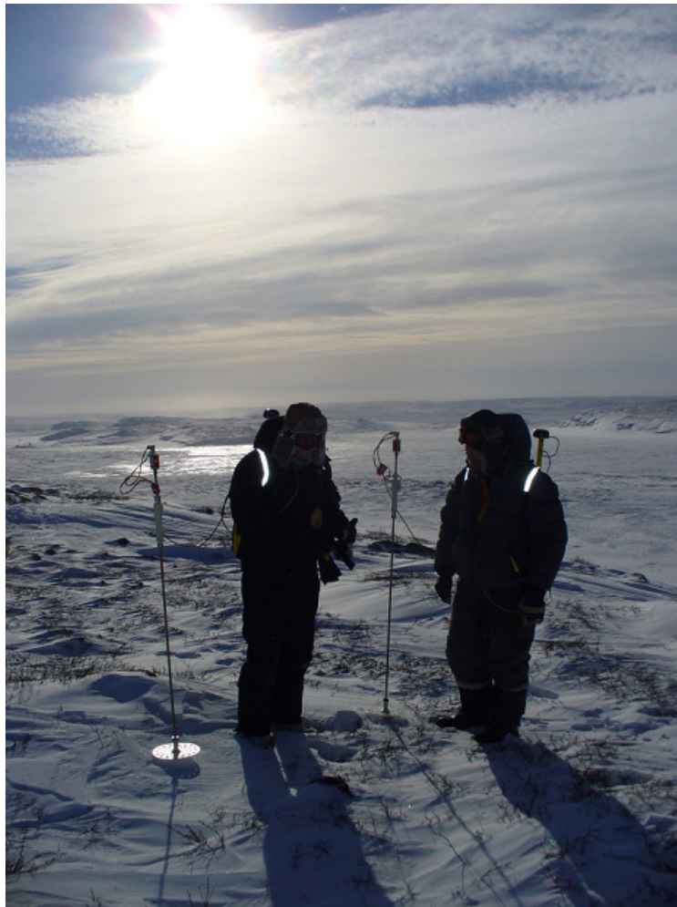
Figure 2.5. Recording snow-depth probe equipped with a GNSS antenna (Canadian Arctic, photo courtesy of Environment and Climate Change Canada)
