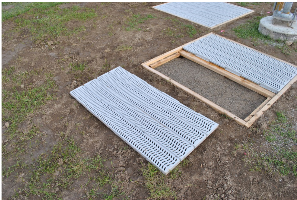
Figure 2.10. Perforated and textured grey plastic target during construction. The panels measuring approximately 1.2 m x 1.2 m are installed on a wooden frame (photo courtesy of Environment and Climate Change Canada).
