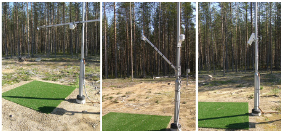
Figure 2.8. Automated sonic snow-depth instrument with steel mounting beam and pole secured with concrete (left), angled mounting beam to reduce collection of snow (middle), and laser instrument mounted at an angle away from the vertical mounting pole (right) (Sodankylä, Finland, photos courtesy of the Finnish Meteorological Institute).
