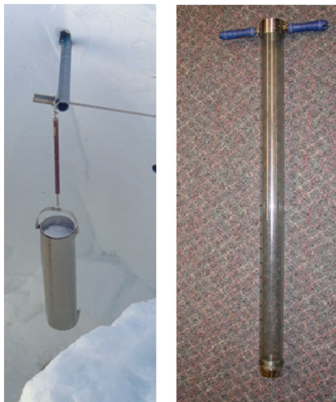
Figure 2.12. A 55 cm-high volumetric sampler being weighed with a spring scale (left, photo courtesy of the WSL Institute for Snow and Avalanche Research SLF, Davos, Switzerland) and a tube snow sampler (right, courtesy of Environment and Climate Change Canada)
