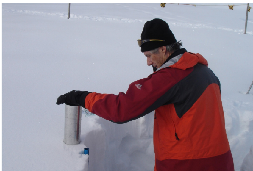
Figure 2.13. Sampling the top layer in a snow pit with an ETH-cylinder sampler (photo courtesy of the WSL Institute for Snow and Avalanche Research SLF, Davos, Switzerland)
