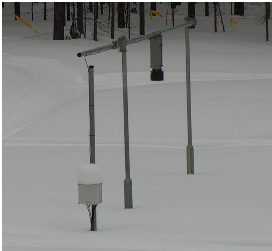
Figure 2.18. Passive gamma radiation SWE instrument (photo courtesy of the Finnish Meteorological Institute)
