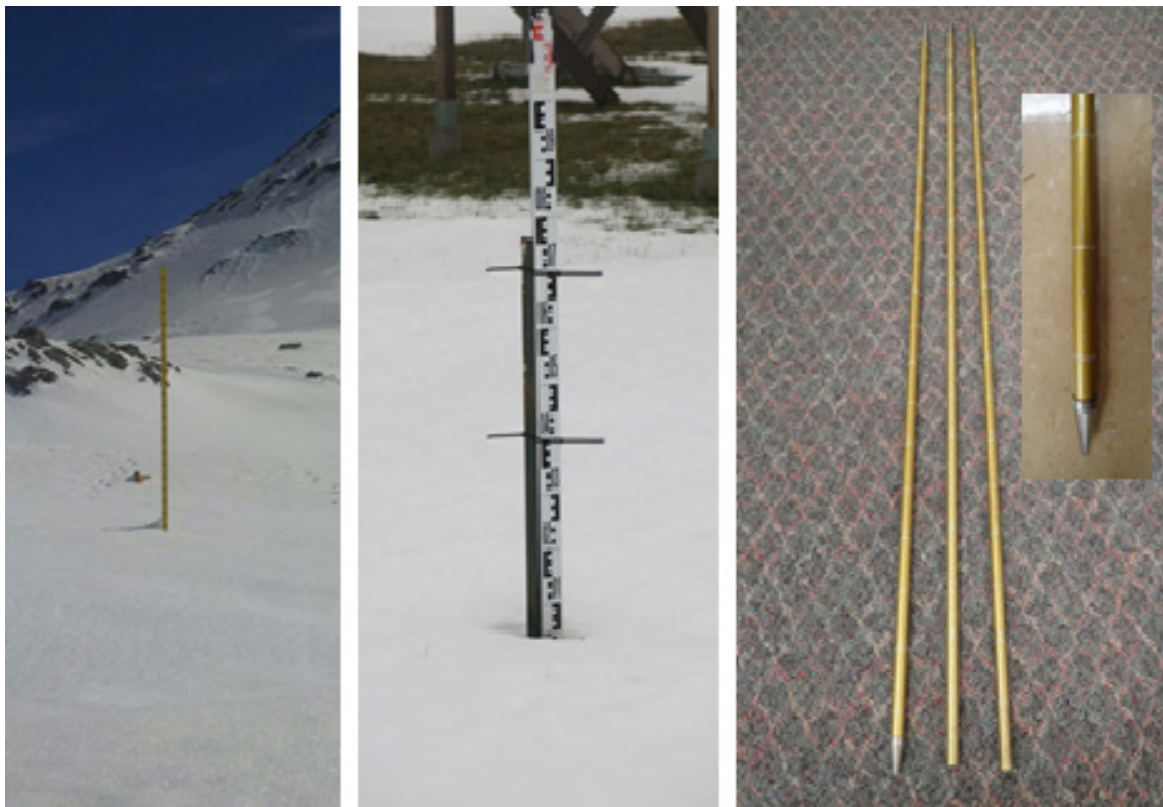
Figure 2.2. Graduated snow stakes in deep alpine snow cover (left, Pyrenees, Spain; photo courtesy of the Spanish State Meteorological Agency) and in shallow snow cover (centre, southern Ontario, Canada; photo courtesy of Environment and Climate Change Canada (ECCC)). An extendible 1 cm graduated snow rod (right, photo courtesy of ECCC)
