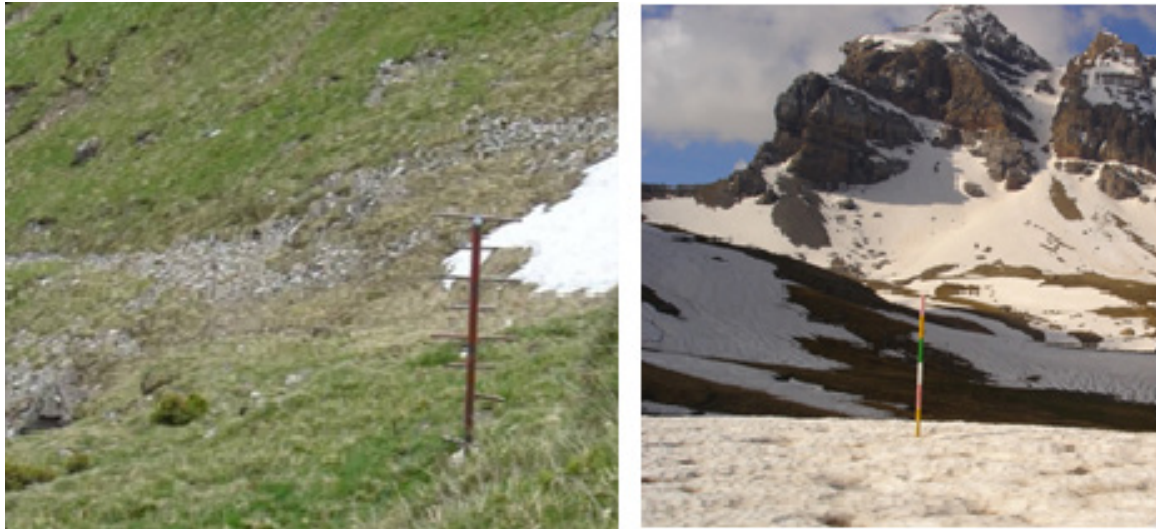
Figure 2.3. Vertical snow stake with horizontal cross arms (left, photo courtesy of the WSL Institute for Snow and Avalanche Research SLF, Davos, Switzerland) and colour coded bands (right, photo courtesy of the Spanish State Meteorological Agency)
