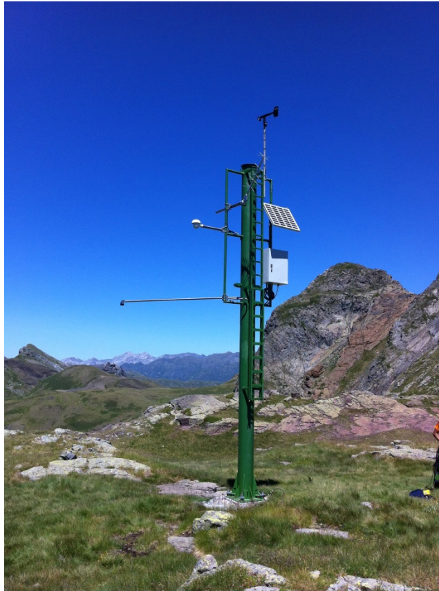
Figure 2.9. Sonic snow-depth instrument (Spanish Pyrenees, photo courtesy of the Spanish State Meteorological Agency)
